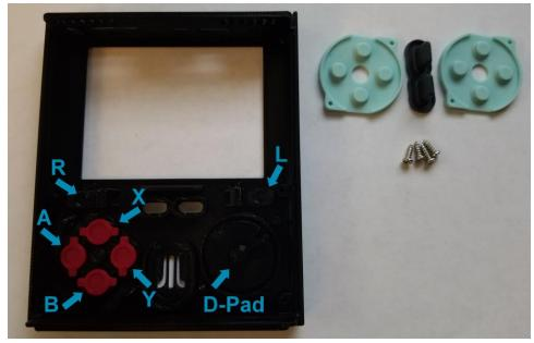
3. Place the silicone membranes into the front shell.
