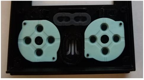
4. Place the speaker inside the pocket between the buttons.
